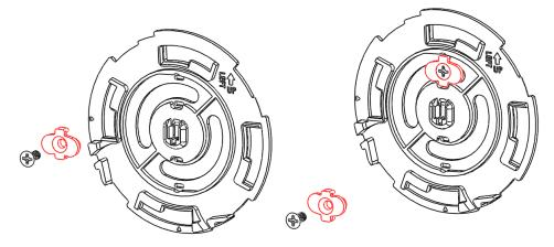
a. For the Swingbolt application, use the retainer type shown above in Red.
