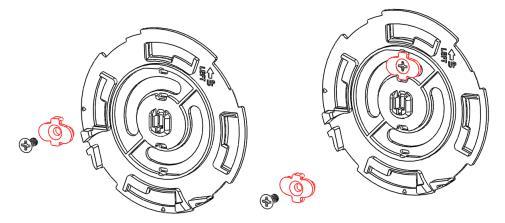
c. For the Swingbolt application, use the retainer type shown above in Red.
