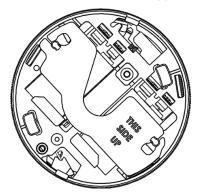
2. Twist the battery cover counterclockwise to detach it from the housing, as shown below:
